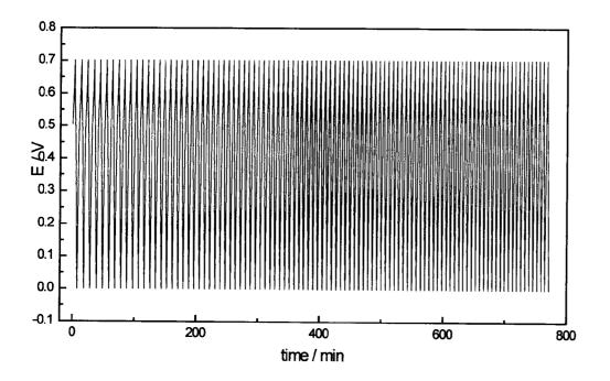
Fig. E3 Charge and discharge cycle of material from Example 1
