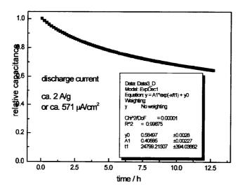
Figure E4. Decay of charge capacity for material from Example 1, versus time over a total of 12 hours.
