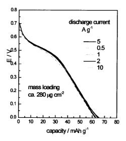
Fig. E2 Electrochemical discharge of materials from Example 1, in 0.1 M HClO<sub>4</sub> aqueous solution.
